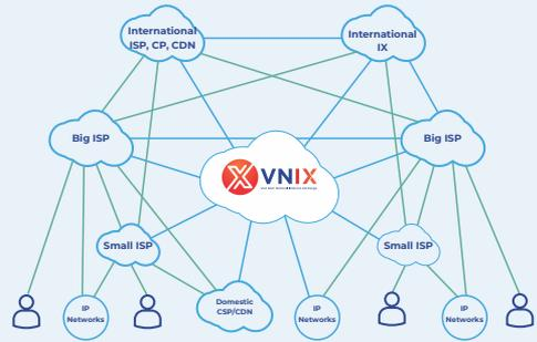
Diagram 4: The architecture model of Viet Nam's Internet connectivity
